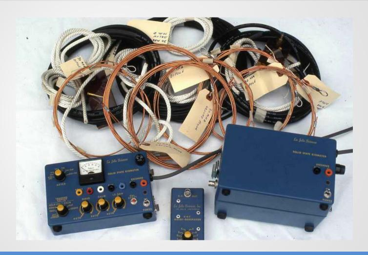
Includes antenna and noise generator for field testing and calibration
