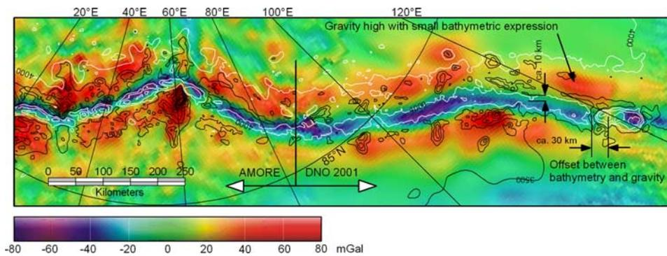
**Figure 3.** Free air gravity compared with bathymetric contours derived from IBCAO Version 2.0. Depth contours deeper than 4000 m are shown in white while shallower are shown in black. There are 500 m depth intervals between contours.
