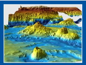
After Malaysia Airlines Flight MH370 mysteriously disappeared over the Indian Ocean in 2014, survey teams generated a digital elevation model of the seafloor to better visualize it in trying to locate the missing plane's wreckage.
