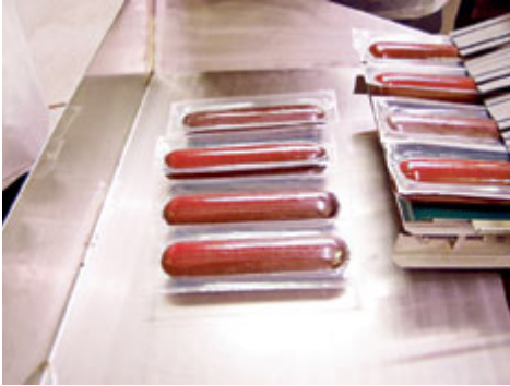
Plates, compartment sizes and films can be changed over in as little as ten minutes.
