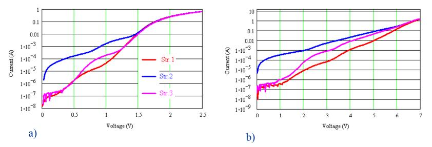
Dark I-V characteristics: a) by-pass diodes; b) solar cells.
