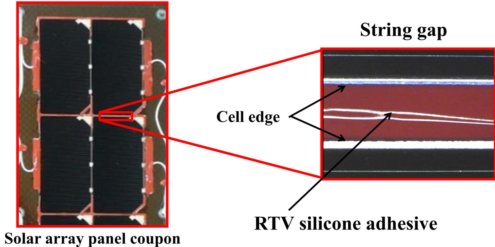
*Effect of aging on Discharge Tolerance of Grouted Solar Array Panels is unclear*
