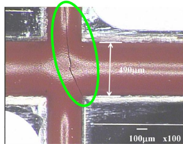
Microscope picture of crack 2
