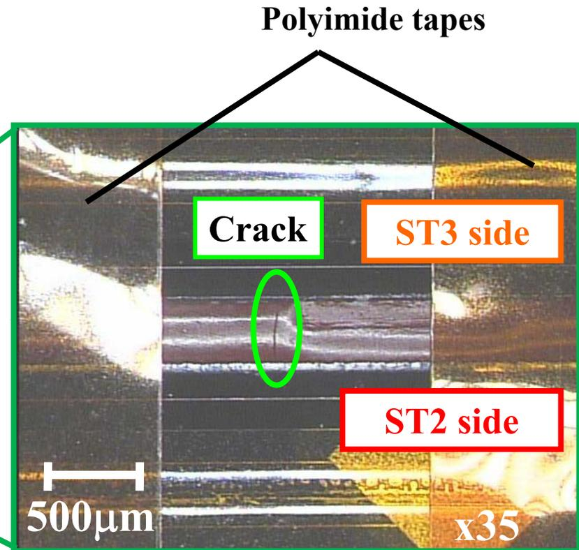
**Electron beam exposed area was limited to the small area which contains crack to confirm secondary arcs occur or not.**
