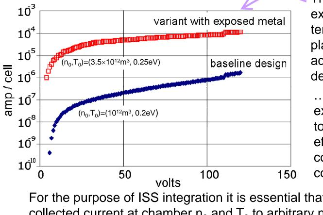
This variant has exposed metal end terminals and plasma state adjusted to higher density conditions.
