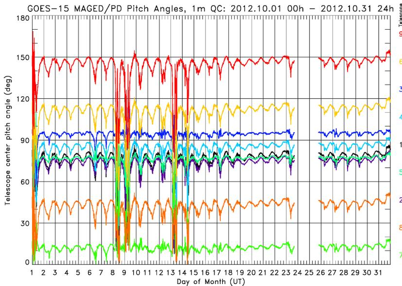
**Figure 3. Pitch angles for MAGE/PD on GOES-15, October 2012. The telescope numbers are given in the right margin, color-coded to match the time series. The spacecraft is upright.**
