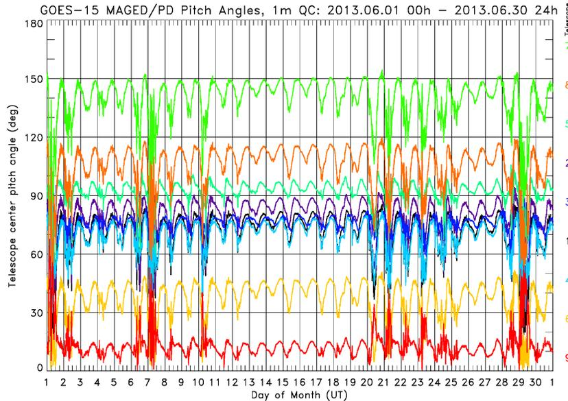
**Figure 4. Pitch angles for MAGE/PD on GOES-15, June 2013. The telescope numbers are given in the right margin, color-coded to match the time series. The spacecraft is inverted.**
