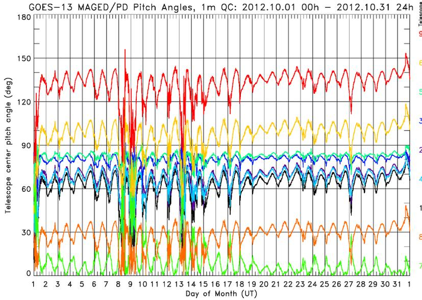
**Figure 2. Pitch angles for MAGE/PD on GOES-13, October 2012. The telescope numbers are given in the right margin, color-coded to match the time series. The spacecraft is upright.**
