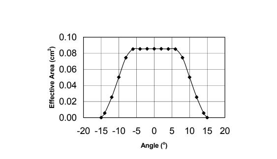
Figure 4-7a. Calculated Angular Response of MAGED Telescopes
