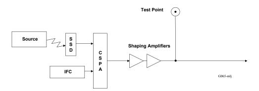
Figure 6-9. EPEAD ASP and Detector Initial Calibration
