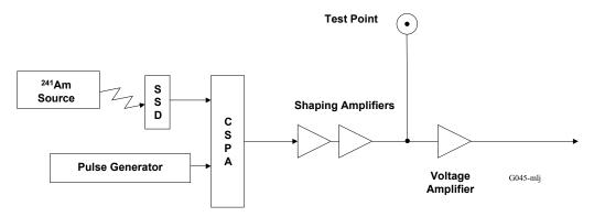
Figure 4-6. MAGED Initial Calibration
