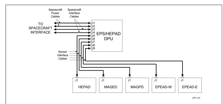
Figure 2-1. EPS/HEPAD Interconnection Diagram
