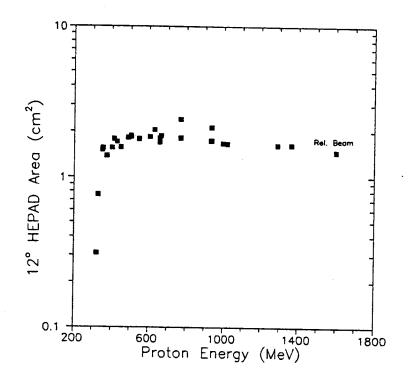
Figure 7-10. Measured HEPAD Area at 12° with Respect to the Beam
