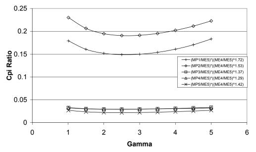
Figure 5-8. Variation of Calculated CPi Constants for MAGPD Electron Response Corrections
