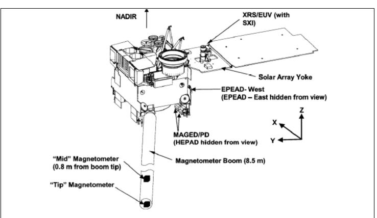
Figure 2-3. Spacecraft View Showing Solar Panels and EPEAD-West Look Direction
