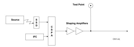
Figure 7-6. HEPAD SSD ASP and Detector Initial Calibration
