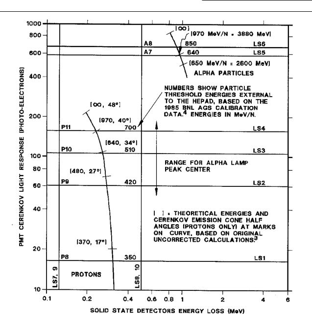
Figure 7-4. HEPAD Telescope Energy Loss Curves
