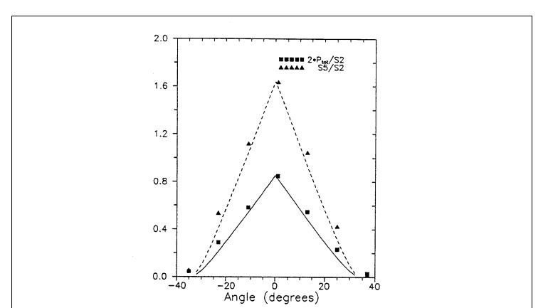
Figure 7-8. Measured and Calculated S5 and P<sub>tot</sub> to Good Proton Ratios Lines show results of calculation using Eq. (7.7)
