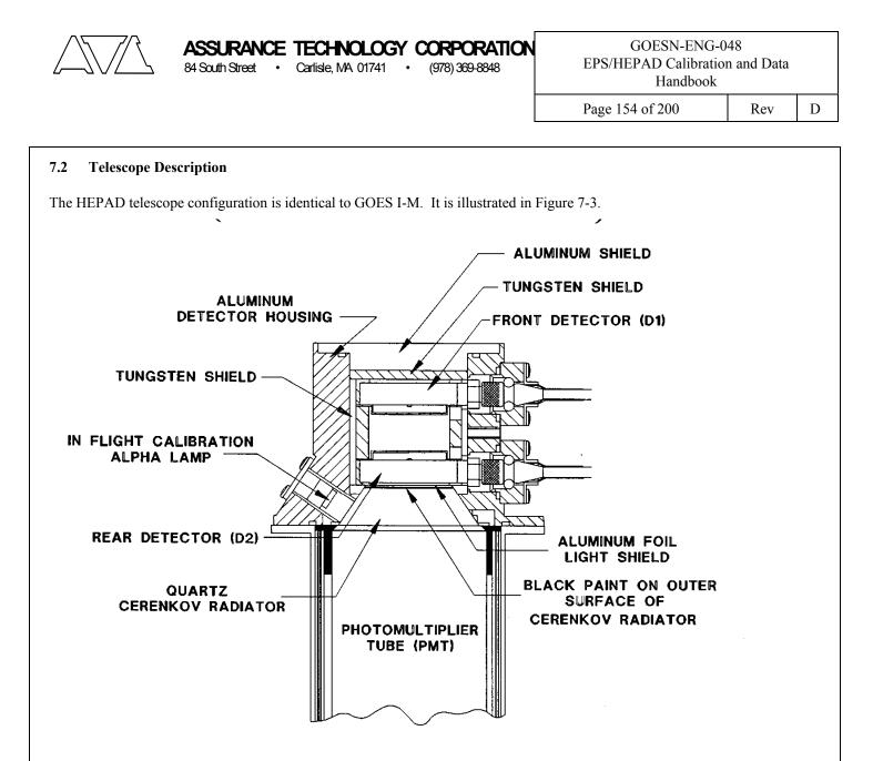
Figure 7-3. HEPAD Telescope Configuration
