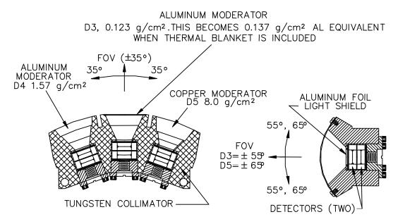
Figure 6-5. EPEAD Dome Configuration
