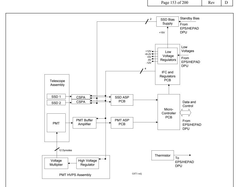
Figure 7-2. HEPAD Block Diagram
