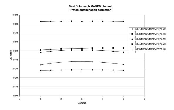
Figure 4-8. Variation of Calculated CEi Constants for MAGED Proton Response Corrections
