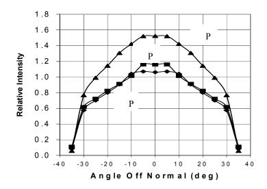
Figure 6-10. Experimental Values of Angular Response for EPEAD Telescope
