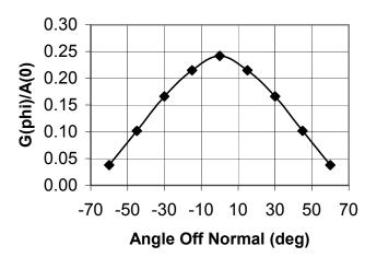
Figure 6-12. Measured Angular Response for D4 at 51 MeV (P5)
