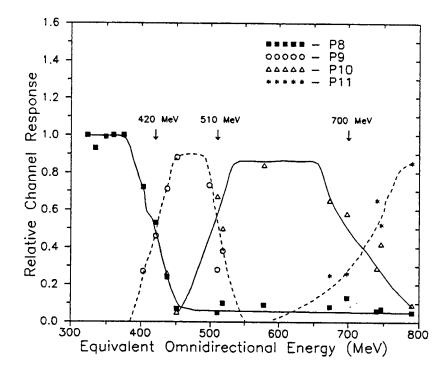
Figure 7-11. Relative Responses of P8, P9, P10 and P11 Channels as a Function of Proton Energy
