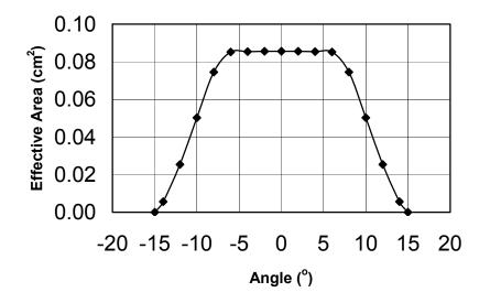
Figure 5-7a. Calculated Angular Response of MAGPD Telescopes
