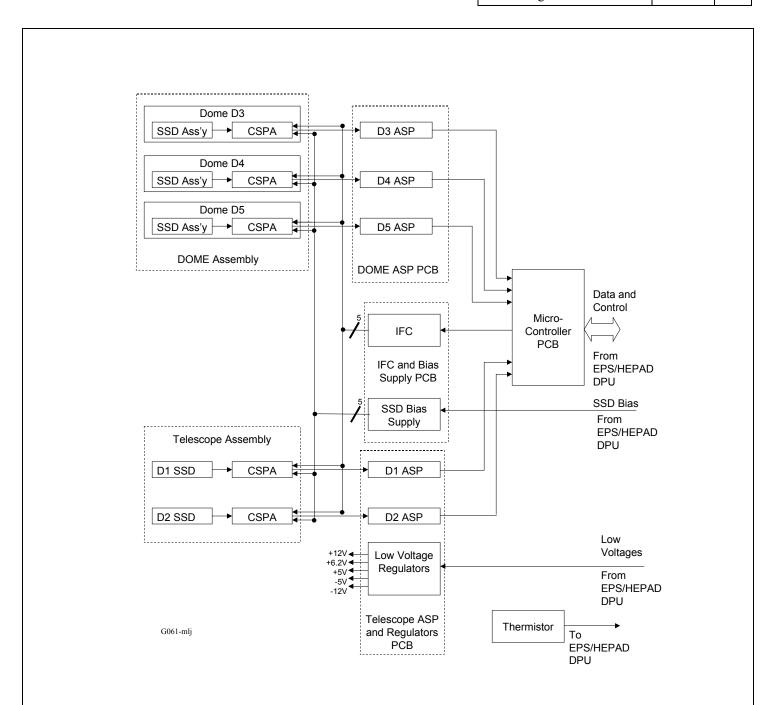
Figure 6-2. EPEAD Block Diagram
