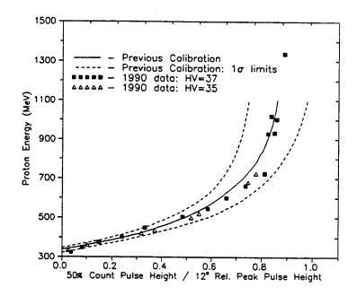
Figure 7-9. Proton Beam Energy Plotted Against the Median Pulse Height from the Photomultiplier Analog Output
