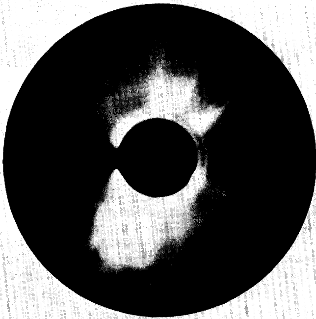
Figure 1-31. White-light photograph of a coronal transient obtained with the High Altitude Observatory white-light coronagraph experiment on Skylab. The black circle is not the sun but the occulting disc of the instrument used to block out photospheric light. The size of its image is two solar radii. This particular transient traveled outward from the sun at about 500 km/s.
